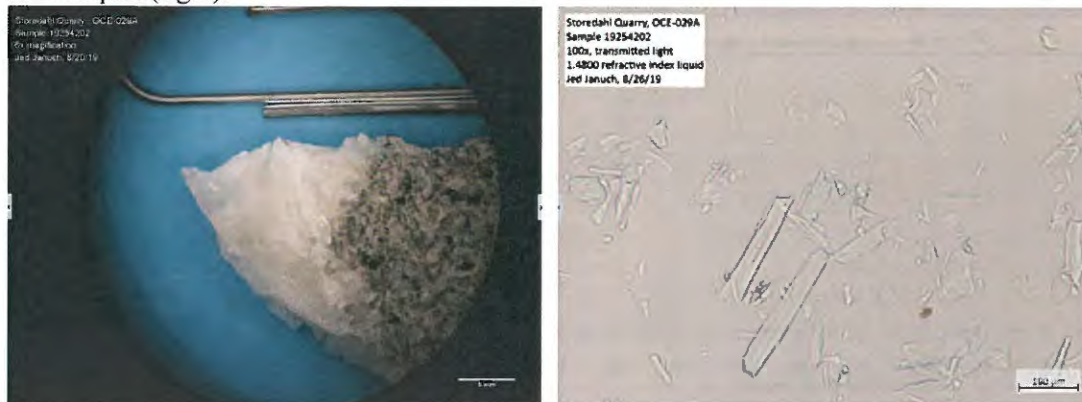
Figure 5 – Stereomicroscope image of white radiating crystals on a basalt rock from sample 19254202 (left) and a polarized light microscope image of the subsample of the crystals mounted in 1.4800 refractive index liquid (right).
